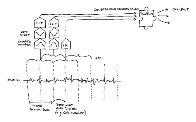
If the plugin requests frequency domain input, each block of audio input is processed by the host using a windowed short time Fourier transform before being supplied to the process function.
