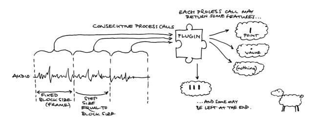
When supplying time domain input, it is most usual for the step size to be equal to the block size as shown above. This means that the plugin is receiving every sample in the audio input exactly once, in a series of contiguous blocks of data.
