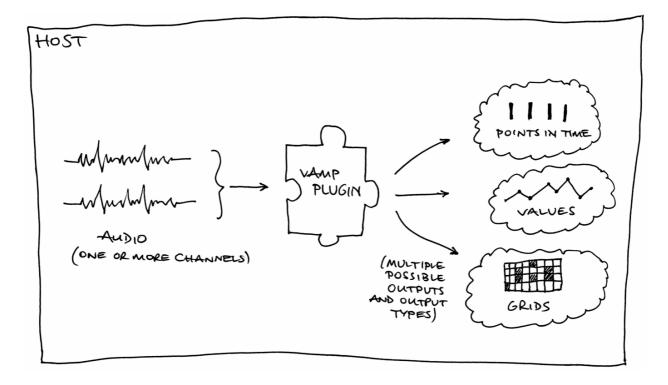
Plugins are not supplied with the whole of their audio input at once, but instead are fed it as a series of short blocks: in this respect they resemble real-time audio processing plugins, but in all other respects they are executed "off-line", meaning that they are not expected to run in real-time and are not obliged to return features as they occur.
